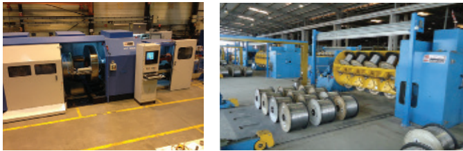
Left: The Setic AST1000R for Cat 8 cables Right: Rigid strander from Pourtier
